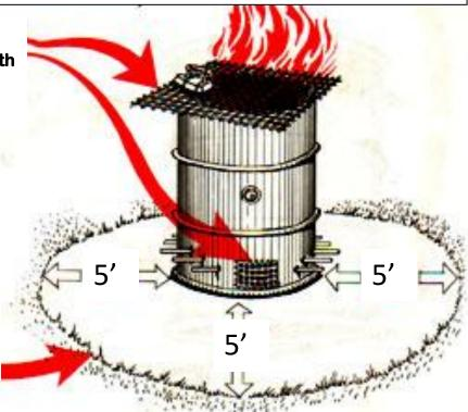
Maintain DRAFT HOLES near the bottom; not larger than 1" inch in diameter.
